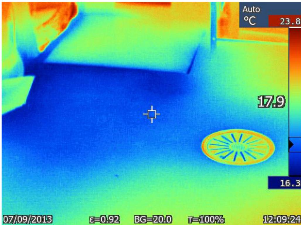
**Figure 41 Infrared image of floor diffuser connected to decentralized air supply units within the concrete**
