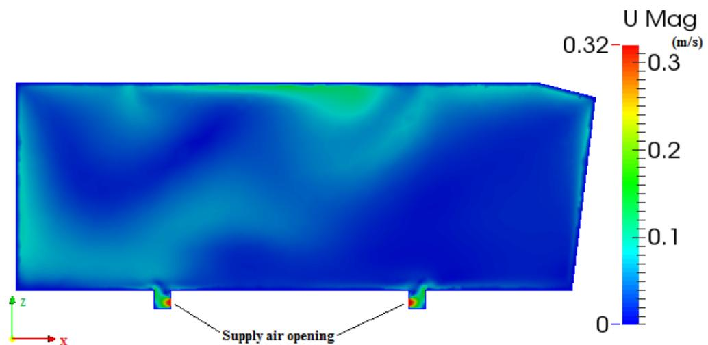
**Figure 68 Predicted air velocity pattern near diffusers**
