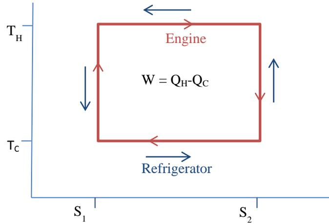
**Figure 27 Ideal Carnot and reverse Carnot cycles in Temperature-Entropy diagram**
