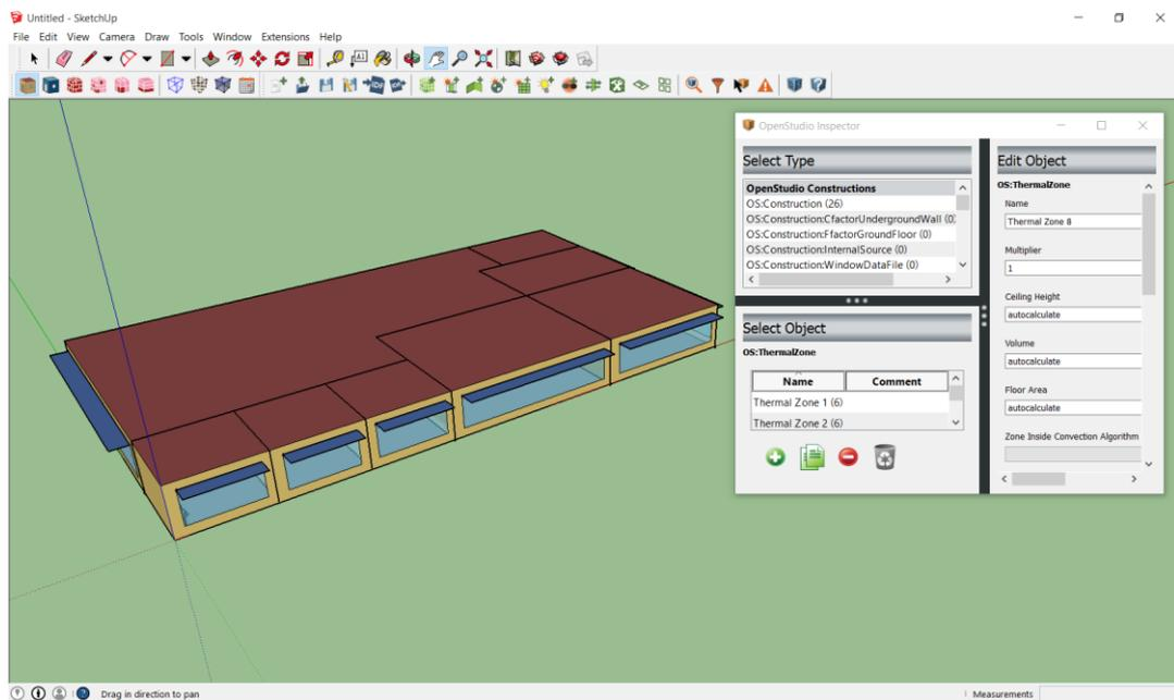
**Figure 29 Three-dimensional geometry of the hypothetical one-storey office building**
