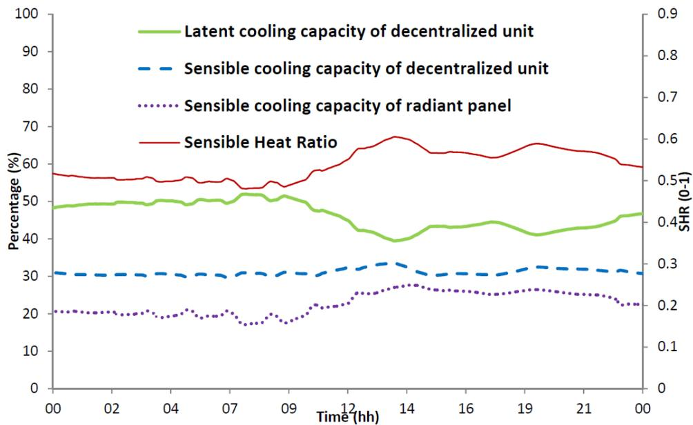
**Figure 53 Ratio of sensible cooling and latent cooling capacities provided by air supply units and panel as well as sensible heat ratio during a typical day**
