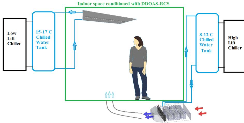
**Figure 17 Schematic diagram of DDOAS-RCP installed in the BubbleZERO**
