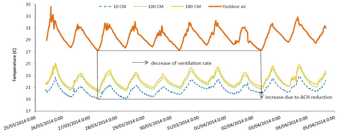
**Figure 51 Measured temperatures at different height levels inside the space and outdoor during reduction of space ventilation rate (0.72 to 0.44 L/s/m<sup>2</sup>)**
