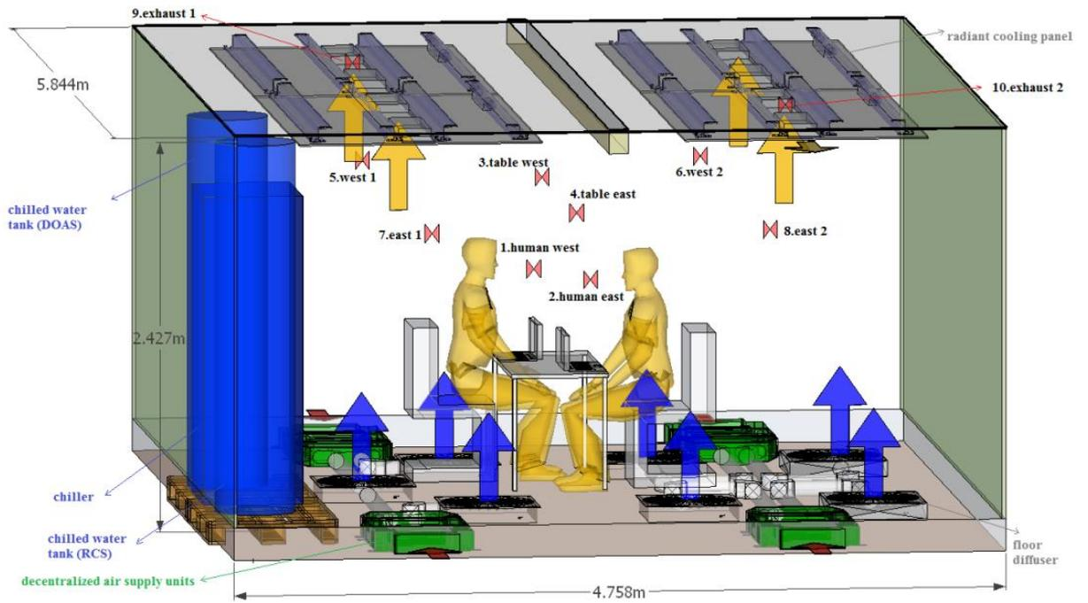
**Figure 22 Setup of ventilation effectiveness experiments including sample points**
