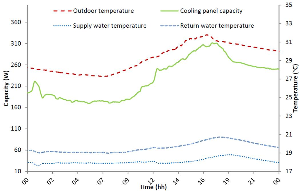
**Figure 47 Daily profile of radiant cooling panel unit capacity caused by fluctuation of outdoor air temperature and supply water temperature**
