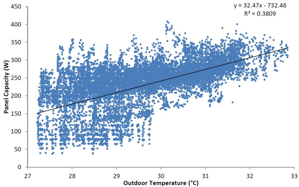
**Figure 48 Pool of sampled radiant panel unit capacity and outdoor temperature**
