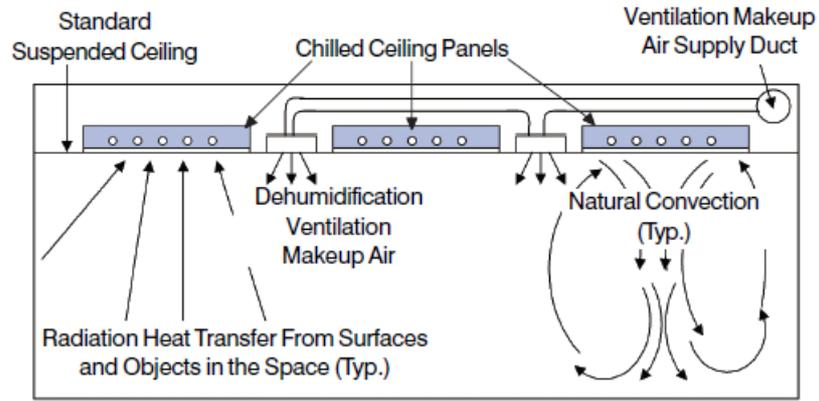
Figure 3 chilled ceiling panel combined with dehumidified ventilation makeup air (Dieckmann et al., 2004)
