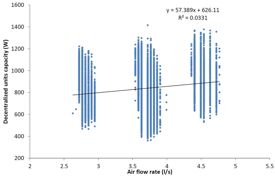
Figure 37 Pool of sampled decentralized air supply unit capacity and air flow rate
