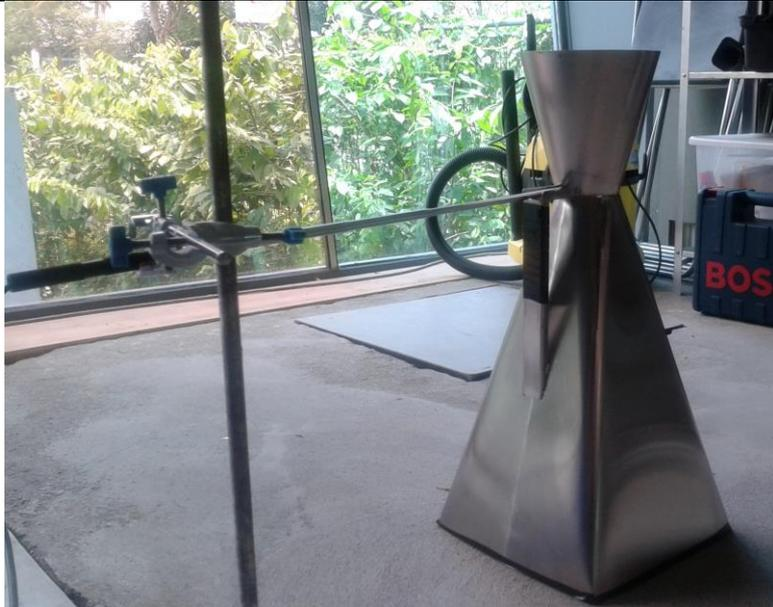
**Figure 21 A custom-designed air flow hood for measurement of air flow rate from diffusers**
