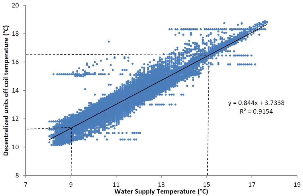
**Figure 36** Pool of sampled decentralized unit off coil temperature and supplied water temperature
