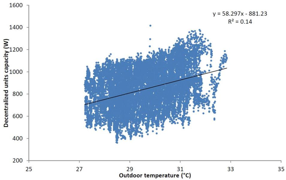
**Figure 40 Pool of sampled decentralized air supply unit capacity and outdoor temperature**
