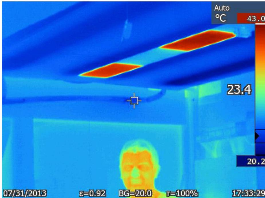
**Figure 46** Infrared image of radiant cooling panel together with human body skin
