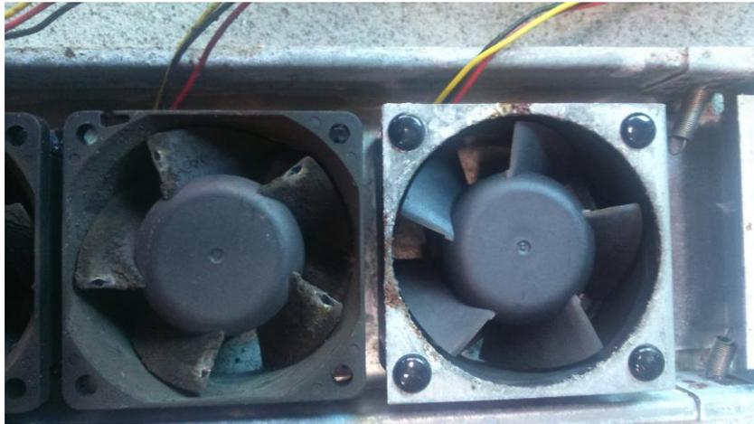
**Figure 42 Erosion of fan blades inside the air supply units after three years of operation**
