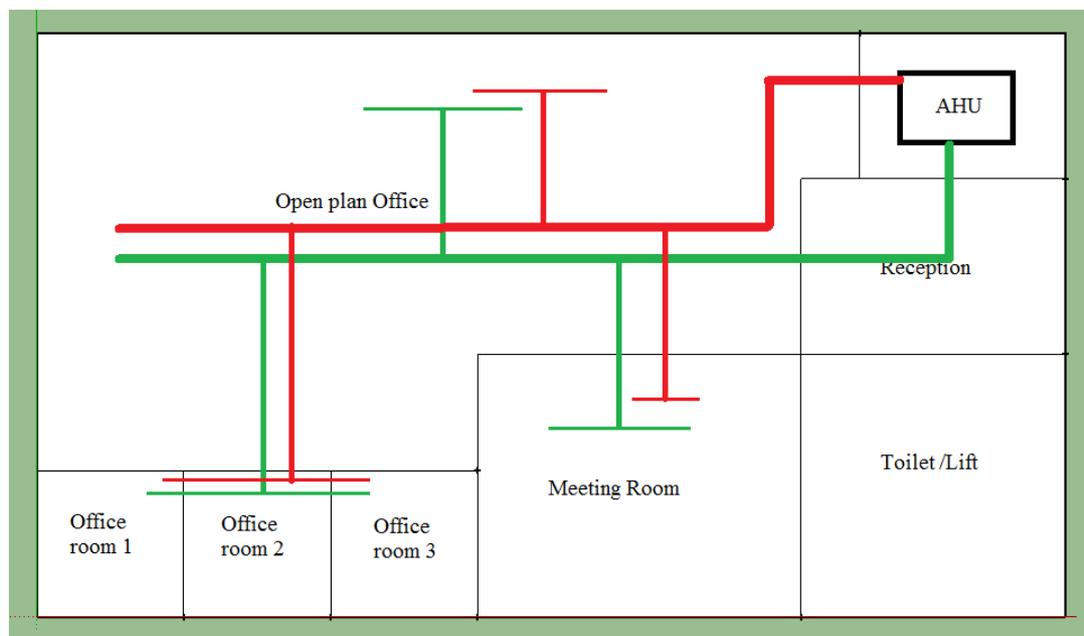
**Figure 30 A typical layout of an all air ACMV system (Green lines are supply ducts, red lines are return ducts)**
