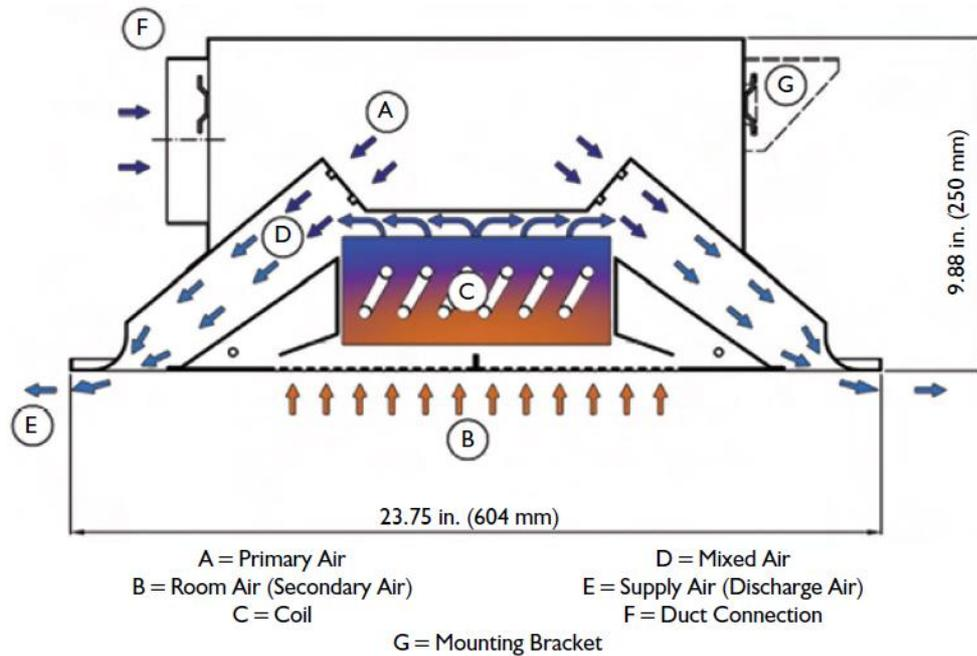
**Figure 6 An active chilled beam in operation (Alexander and O'Rourke, 2008)**
