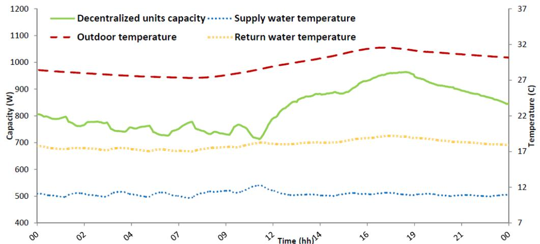
**Figure 34 Daily profile of decentralized units' capacity caused by fluctuation of outdoor air condition and supply water temperature**
