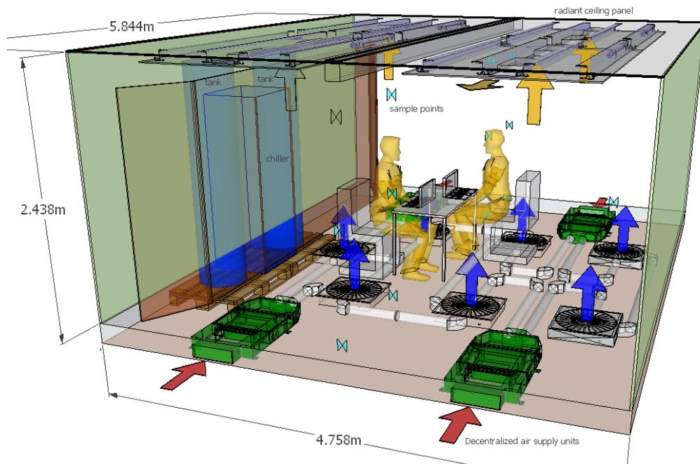
**Figure 18 Illustration of sample points and seated occupants during experiments**
