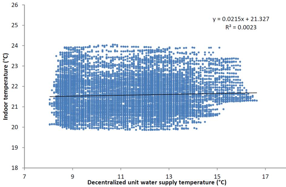
Figure 56 Pool of sampled indoor temperature and decentralized unit water supply temperature
