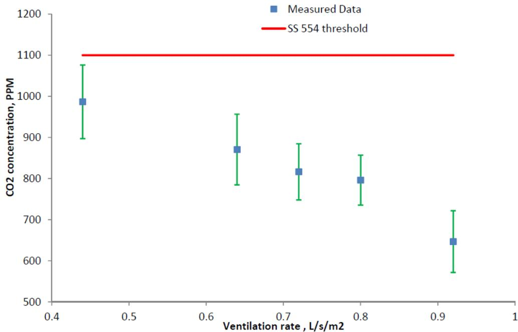
**Figure 60 Carbon dioxide concentrations for five considered ventilation rates and threshold value set by local standard SS 554**
