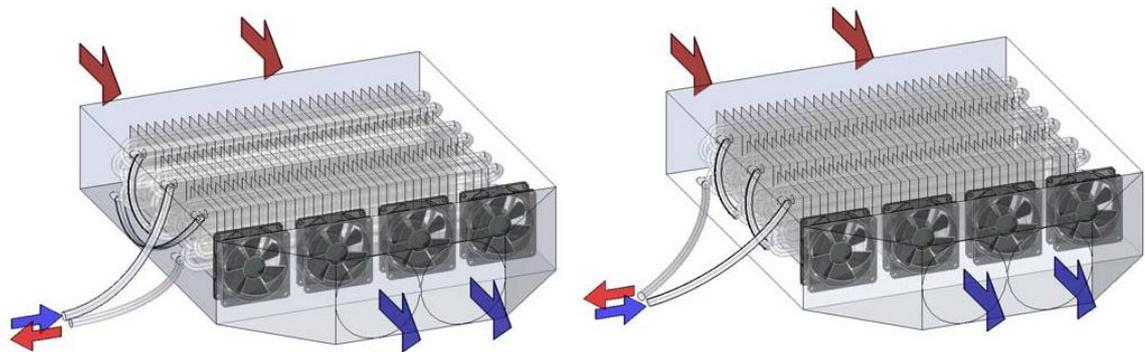
**Figure 32 Two arrangements (left-arrangement A, right-arrangement B) of three heat exchangers inside the units**
