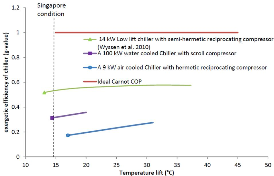
**Figure 78 Exergetic efficiency of the low lift chiller and the two typical air cooled / water cooled chiller at evaporative temperature of 15 °C**
