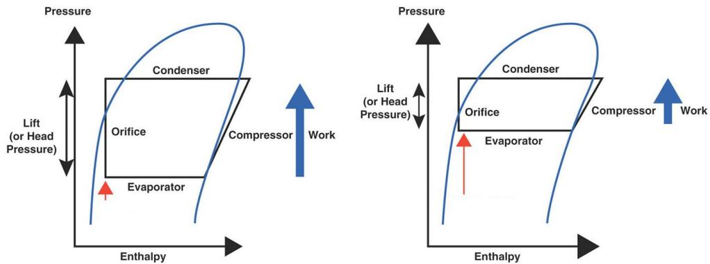
**Figure 12 Impact of raising the evaporative temperature on refrigeration cycle diagram (Doyon, 2008)**
