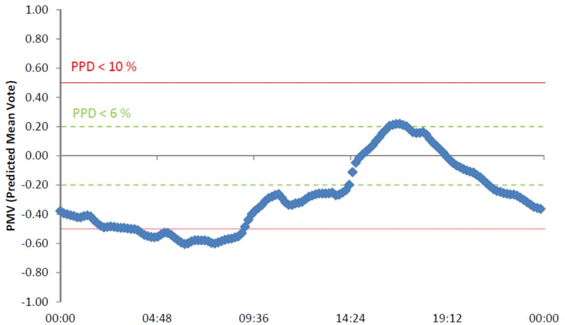
**Figure 59 Calculated daily PMV in the BubbleZERO under fixed operational settings of system**
