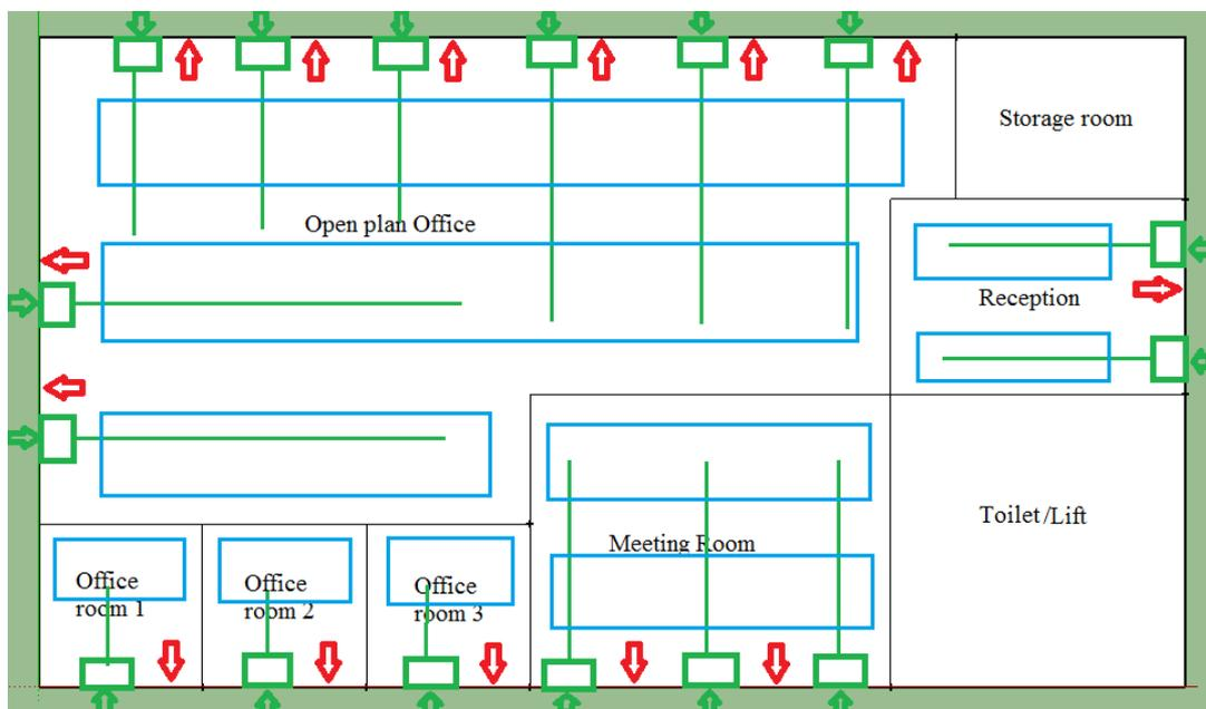
**Figure 31 A suggested ACMV layout for implementation of DDOAS-RCP in the building (green boxes are decentralized units, blue boxes are radiant panels, green lines are supply ducts, green arrows are outdoor air points and red arrows are exhaust points)**
