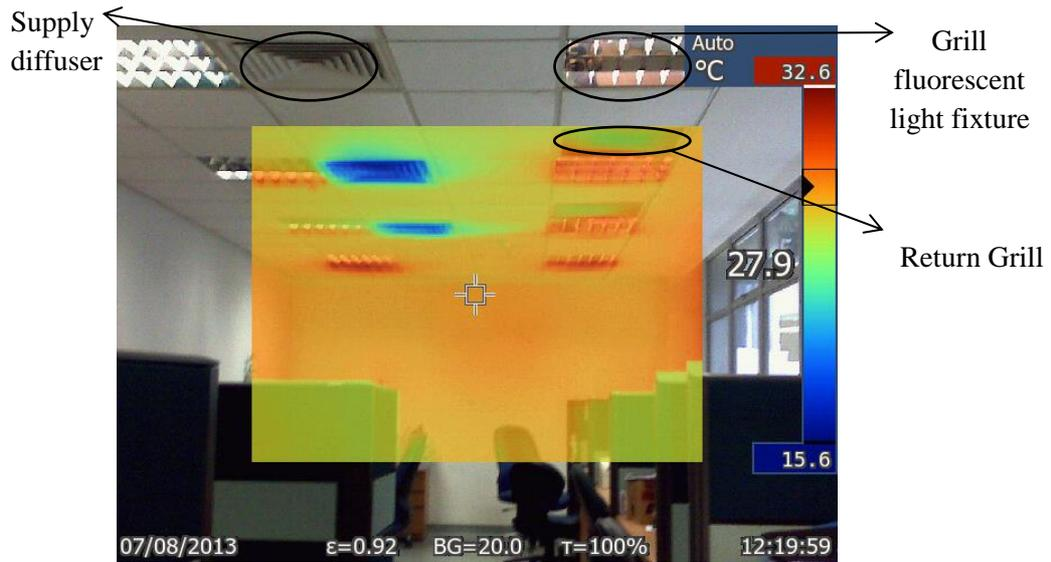
**Figure 8 Infrared image of an interior office space with central all air VAV system**
