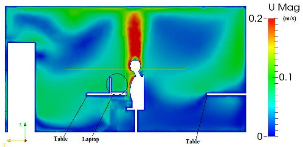
Figure 70 Predicted air velocity pattern near human body
