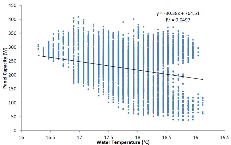
**Figure 49 Pool of sampled radiant panel unit capacity and water supply temperature**
