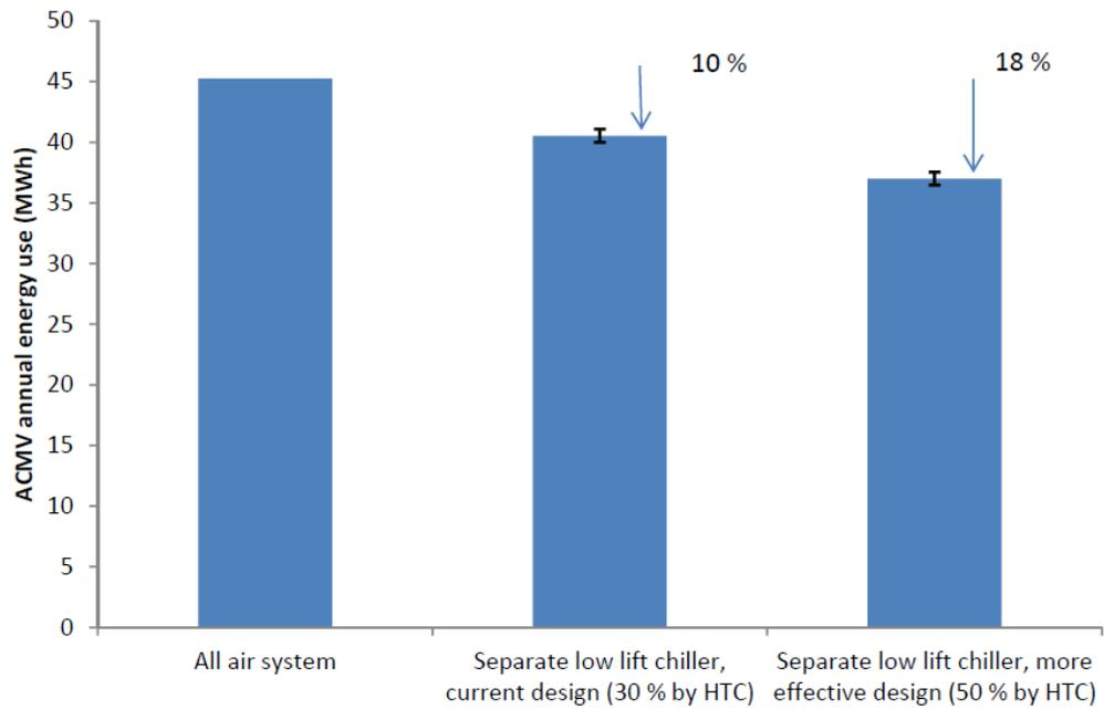
**Figure 80 predicted annual energy saving of high temperature cooling for the hypothetical one-storey building**
