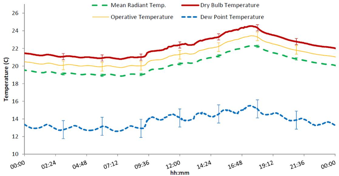
**Figure 52 Variation of dry bulb, mean radiant, operative and dew point temperatures during a typical day**
