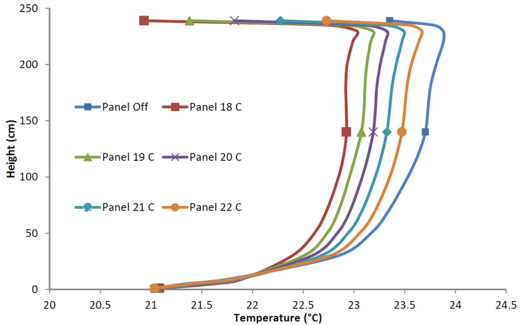
**Figure 74 Predicted air temperature for various panel surface temperatures under area-weighted average uncooled surfaces temperature (AUST) of 23.5 °C**
