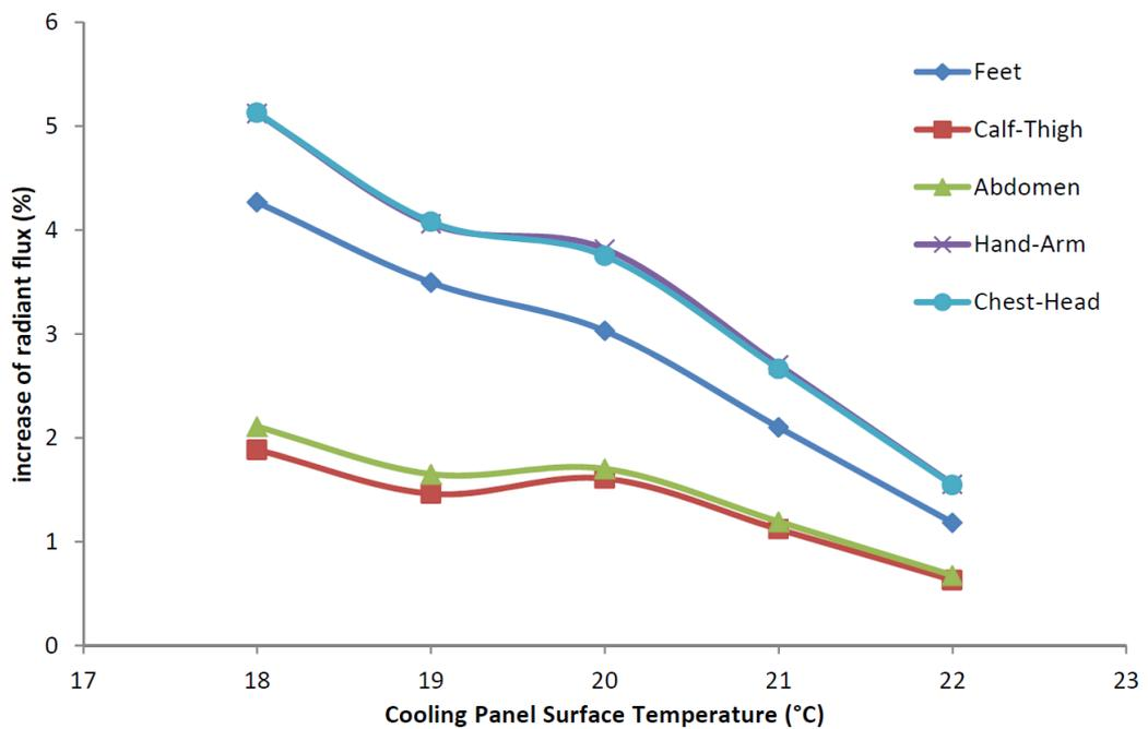
**Figure 75 Increase in radiant flux compared to panel off scenario for different human body segments**
