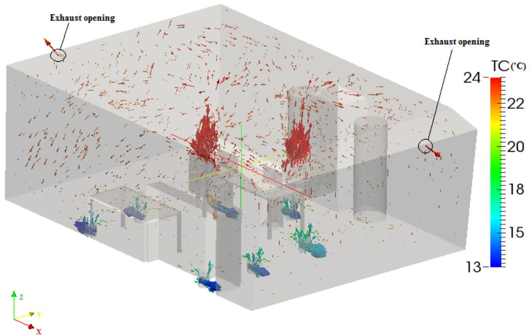
**Figure 72 Velocity vectors in the BubbleZERO scaled by velocity magnitude and colored by temperature**
