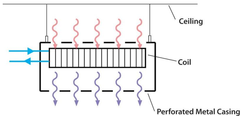
Figure 5 A passive chilled beam in operation (Rumsey and Weale, 2007)
