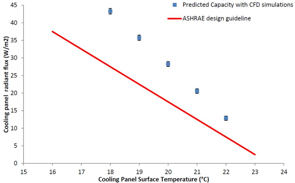
**Figure 73 Radiant flux of cooling panel for various panel surface temperatures under area-weighted average uncooled surfaces temperature (AUST) of 23.5 °C**
