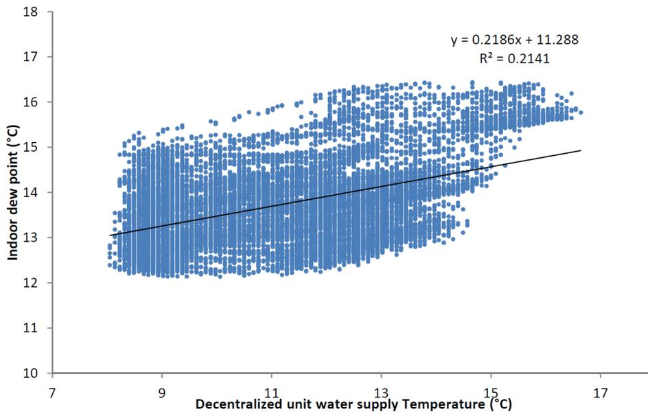
**Figure 57 Pool of sampled indoor dew point temperature and decentralized unit water supply temperature**
