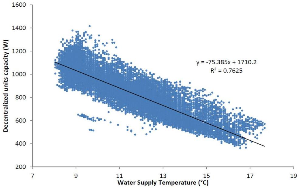
**Figure 35** Pool of sampled decentralized unit capacity and supplied water temperature
