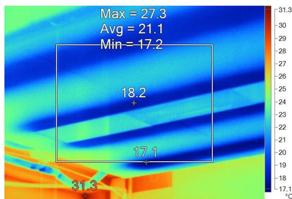
Infrared image of radiant panel
