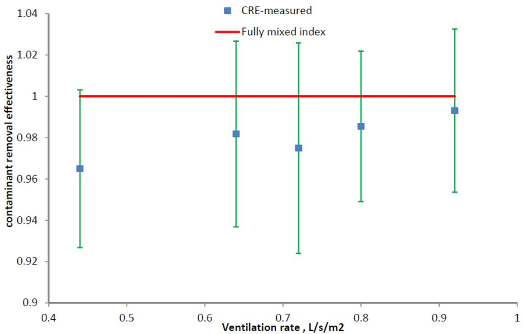
**Figure 66** Calculated contaminant removal effectiveness for five considered ventilation rates
