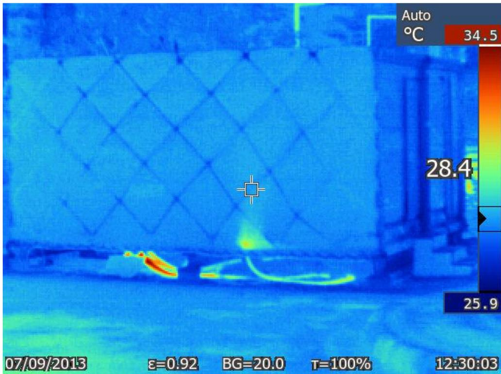
Figure 15 Infrared image of the BubbleZERO laboratory located in outdoor space (red points below the container are the air compressor and its connections to the inflated air skin façade)
