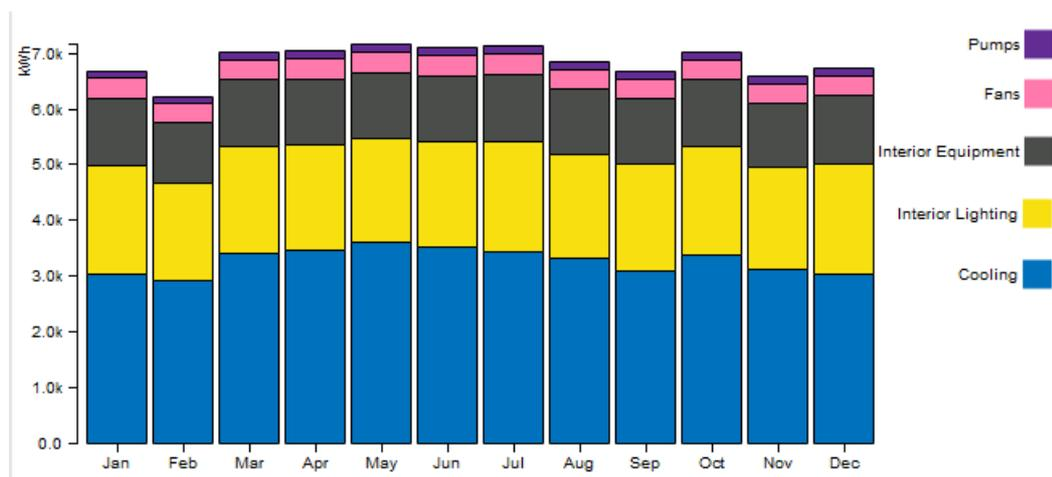
**Figure 79 Monthly electricity consumption of the simulated one-storey building for different stacks of building services**
