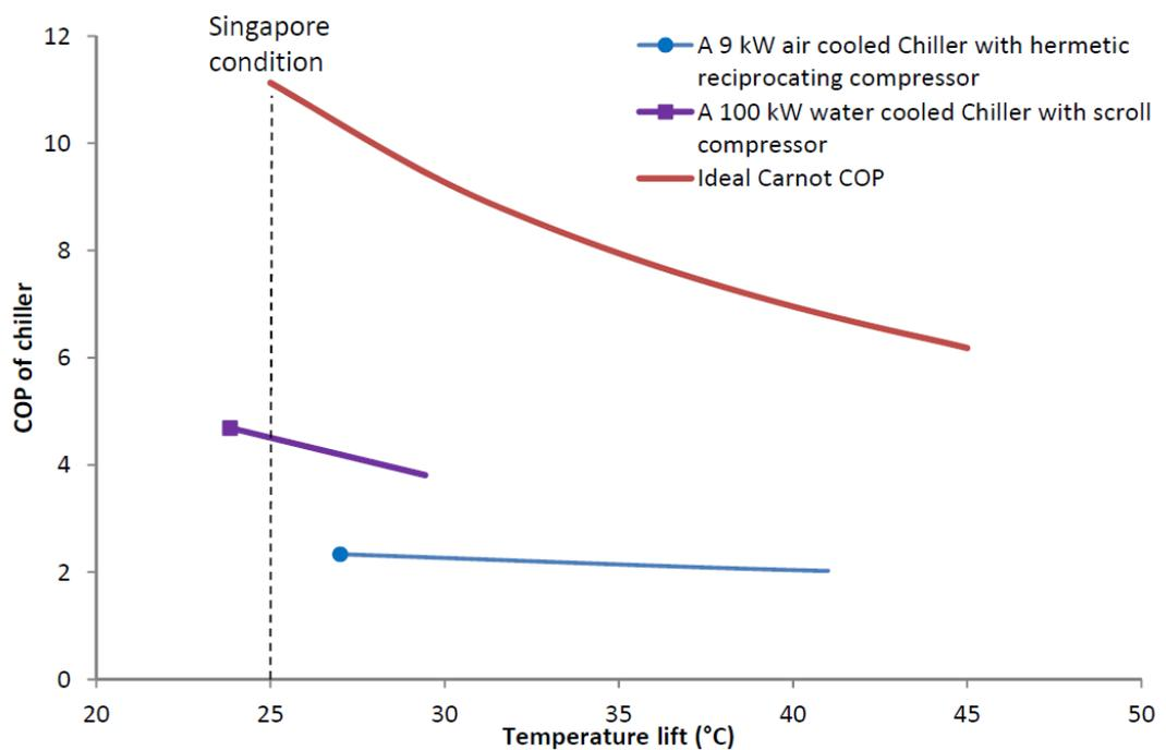
**Figure 76 COP of ideal Carnot cycle and a small size chiller at evaporative temperature of 5 °C**
