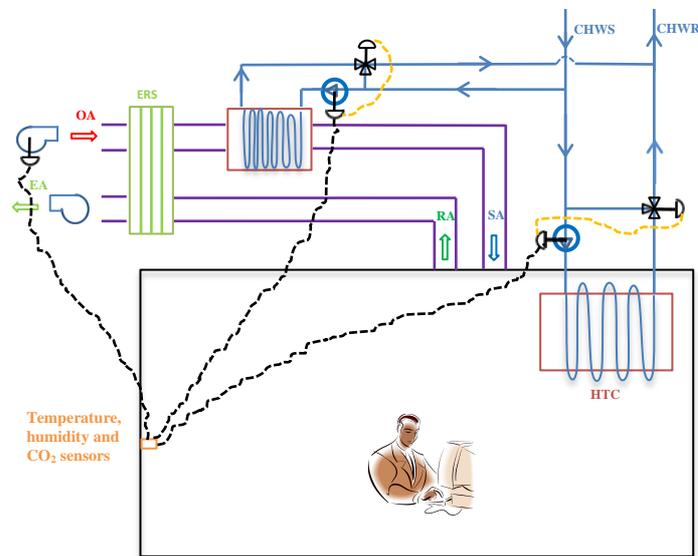
**Figure 81 selected design and control strategies scheme for application of high temperature cooling with one chiller**
