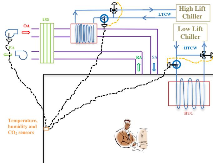
**Figure 82 Selected design and control strategies for application of high temperature cooling with two separate chillers**
