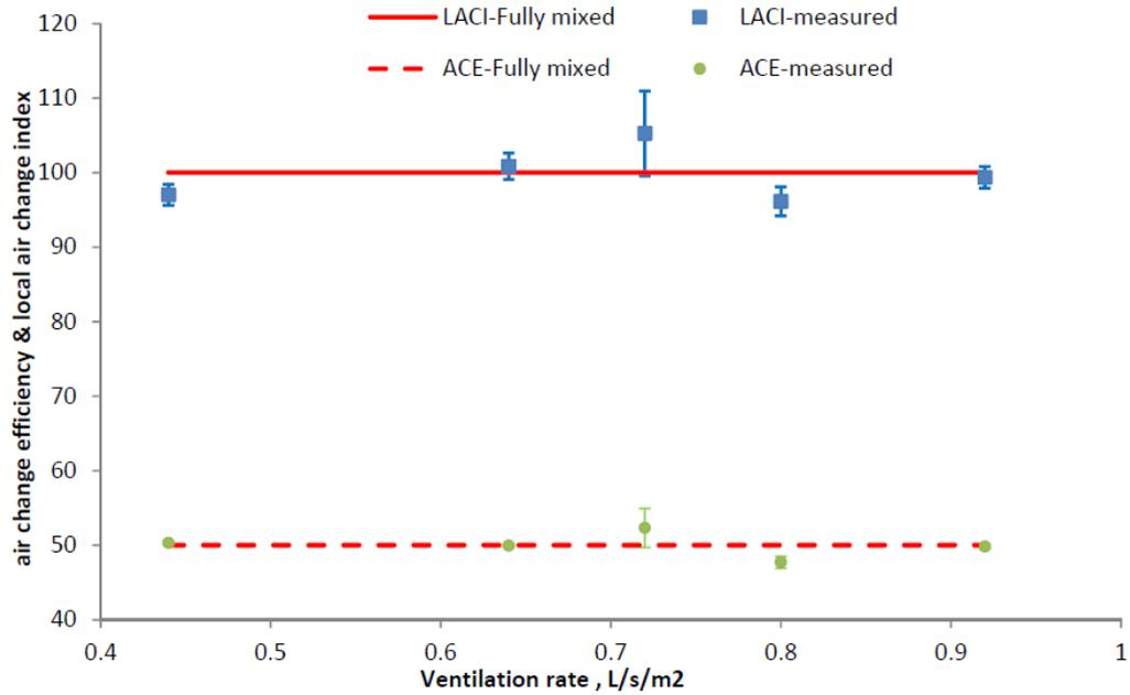
**Figure 65** Calculated air change efficiency (ACE) and local air change index (LACI) for five considered ventilation rates
