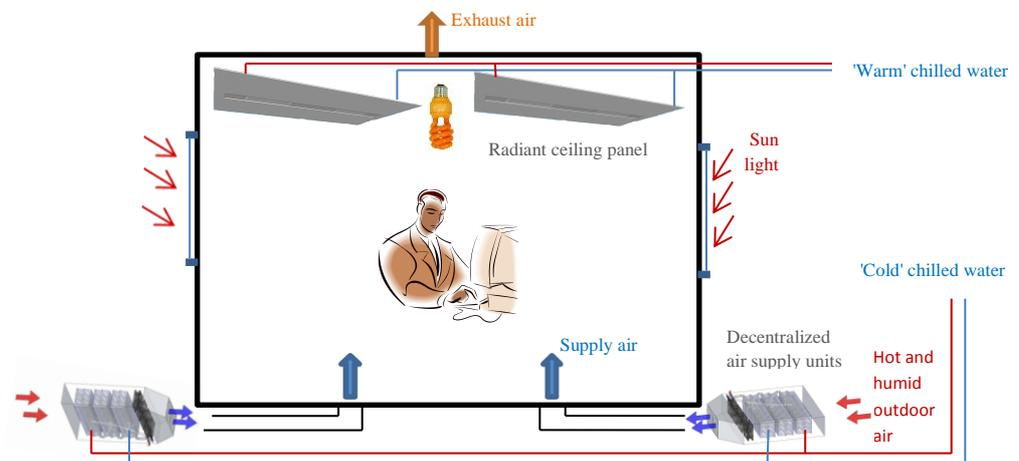
**Figure 10 Schematic of decentralized DOAS combined with radiant ceiling panel**
