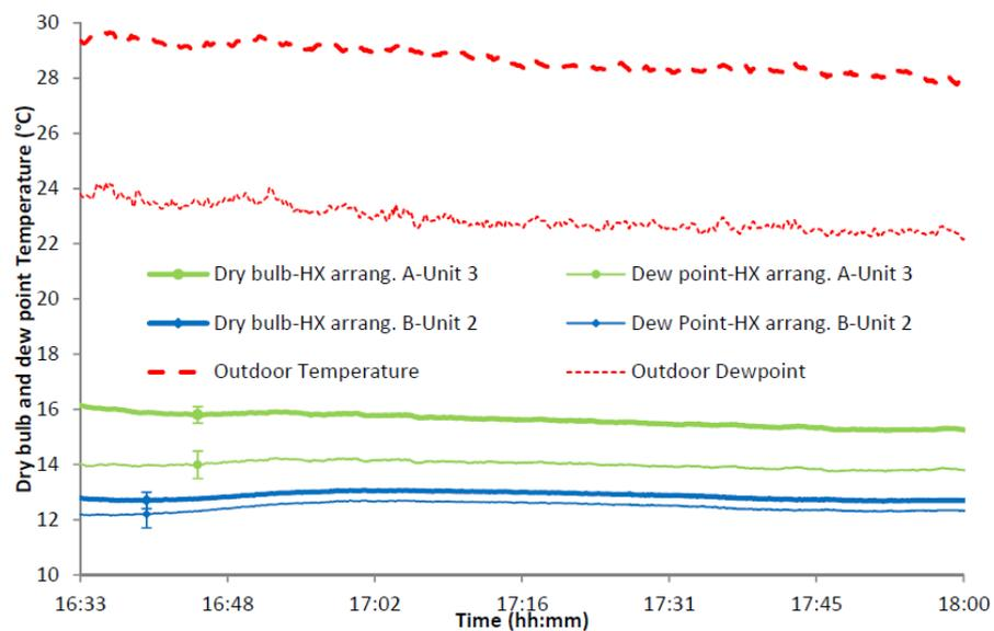
**Figure 33 Off coil air condition of decentralized air supply units with different heat exchanger (HX) arrangements**
