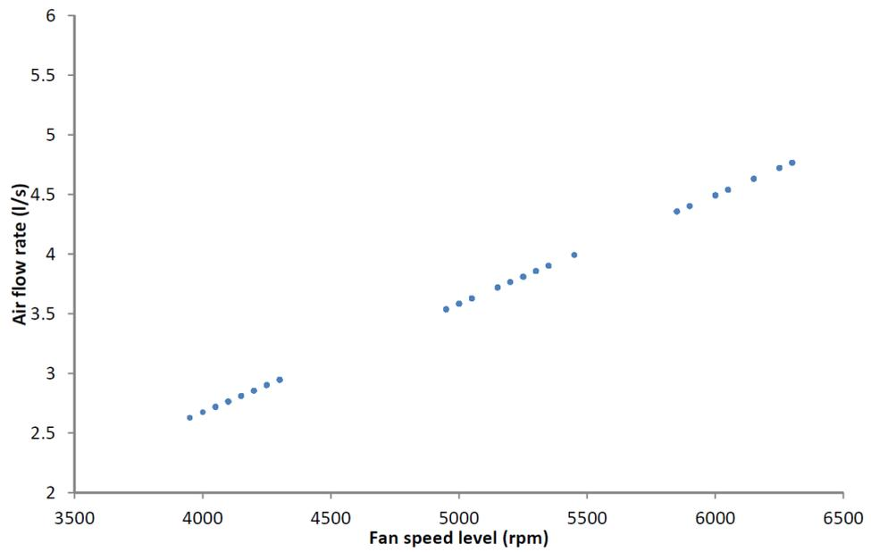
**Figure 39 Air flow rate of unit in terms of fan speed level**
