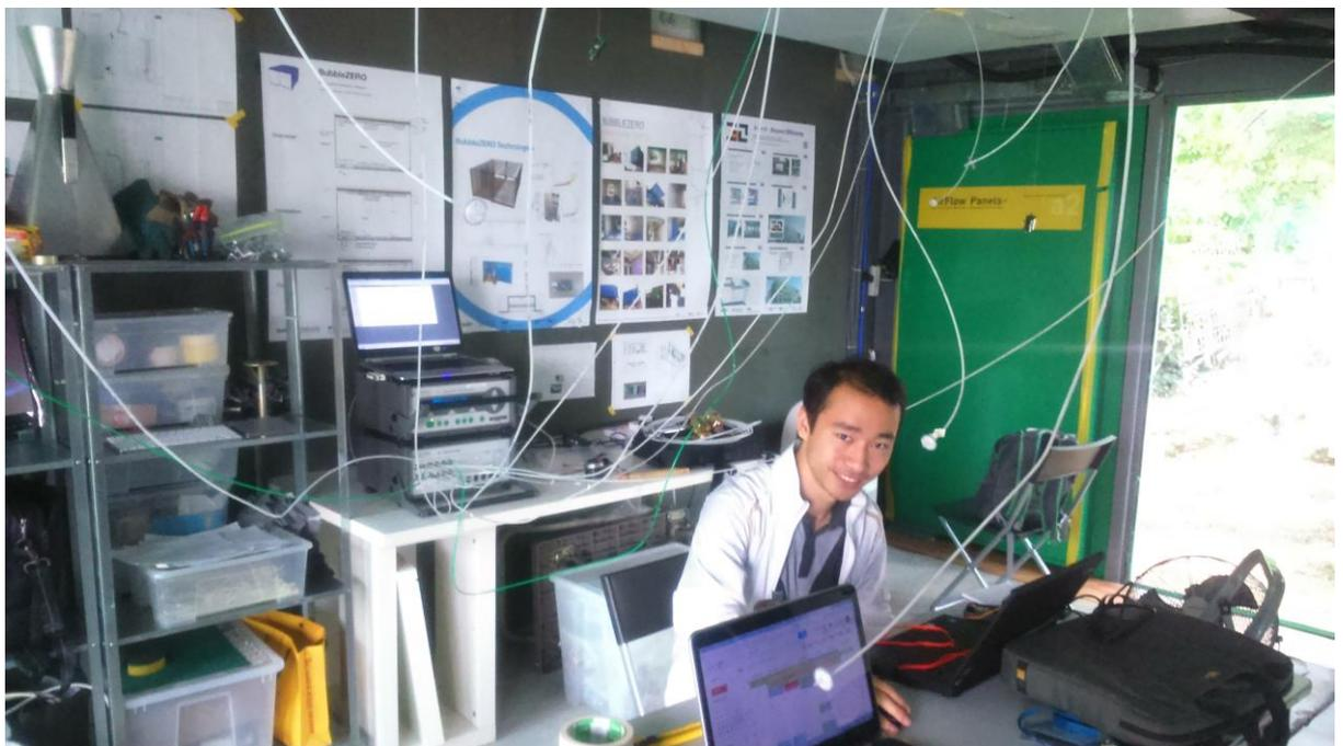
**Figure 23 Sample points placed in different locations inside the BubbleZERO for ventilation effectiveness analysis of DDOAS-RCP**
