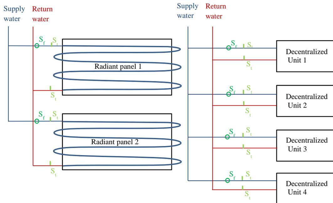
**Figure 20 Schematic of sensor locations and types on DDOAS-RCP components**
