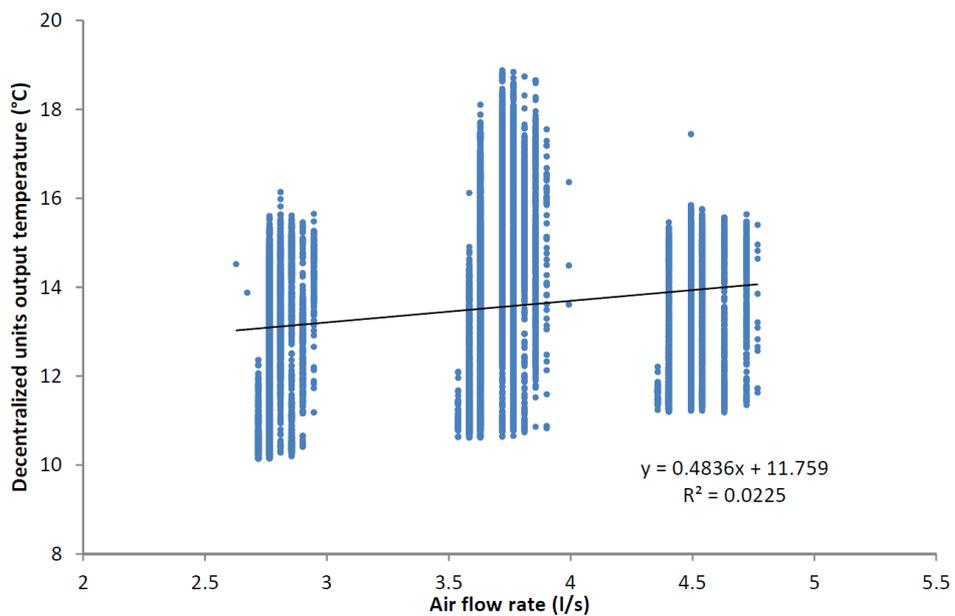
Figure 38 Pool of sampled decentralized air supply unit off coil temperature and air flow rate
