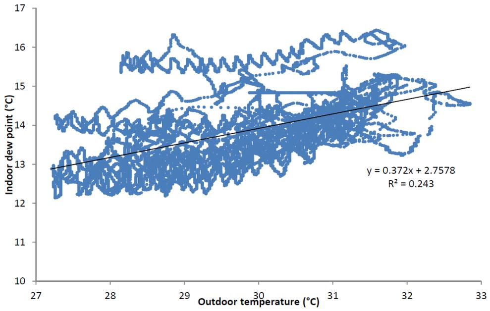
Figure 55 Pool of sampled indoor dew point temperature and outdoor temperature
