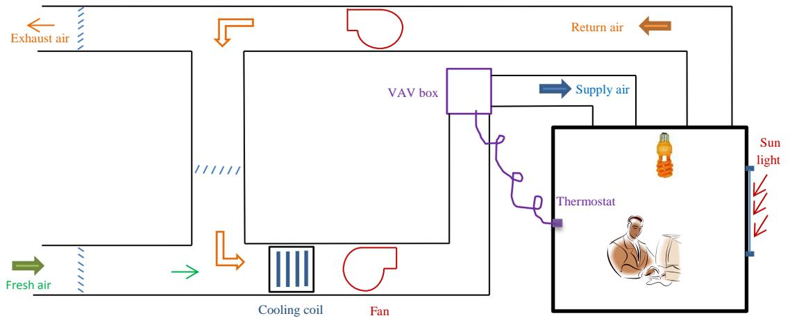
**Figure 7 Schematic of VAV system without reheat in Singapore office buildings**
