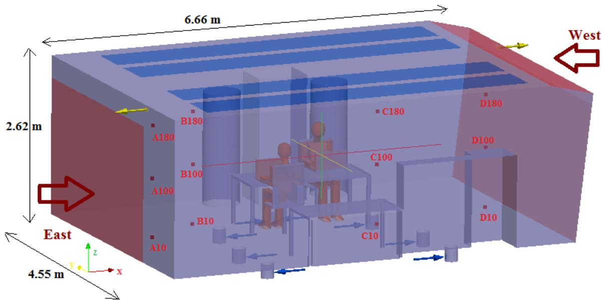
**Figure 24 Sample points at different locations and heights inside the BubbleZERO**
