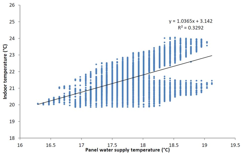
**Figure 58 Pool of sampled indoor temperature and panel water supply temperature**
