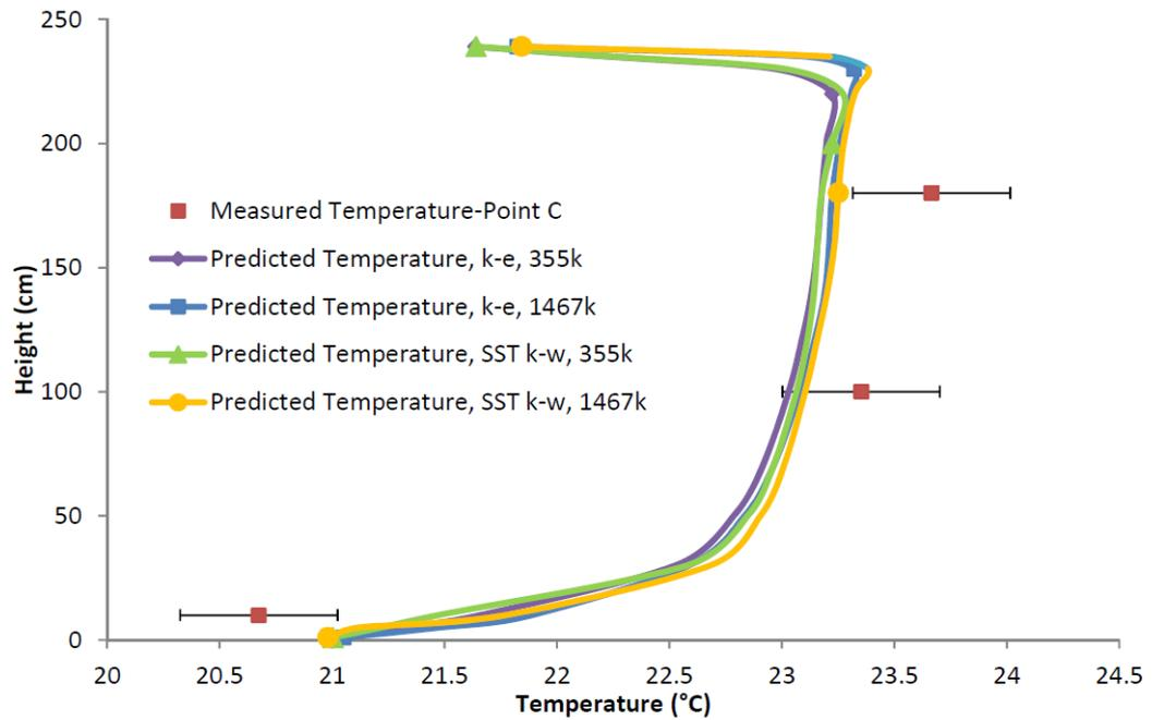
**Figure 67 Predicted thermal stratification with different mesh densities and turbulence models vs measured data at point C in centre of laboratory**
