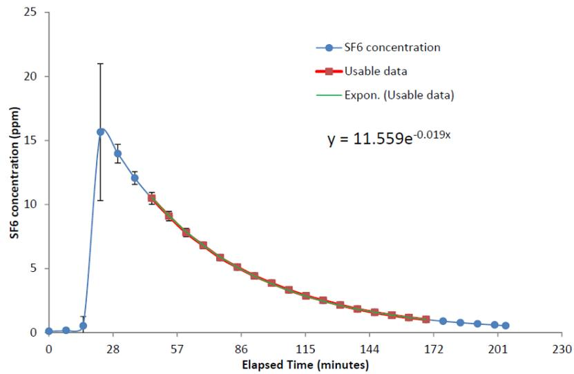
**Figure 63 Measured SF<sub>6</sub> concentration and interpolated curve for a SF<sub>6</sub> step down tracer gas decay test**
