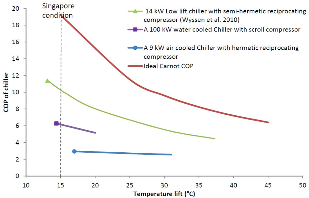
**Figure 77 COP of ideal Carnot cycle, low lift chiller and two typical air cooled/water cooled chillers at evaporative temperature of 15 °C**
