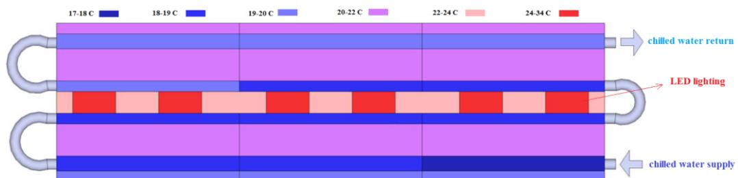
**Figure 45** Measured temperature distribution on the ceiling panel surface
