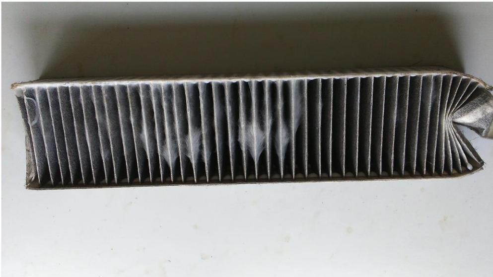
**Figure 43 Erosion of filter sheet inside the air supply units after one year of operation**
