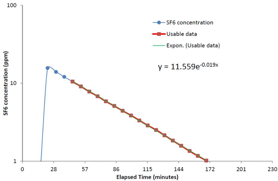
**Figure 64 Measured SF6 concentration and interpolated curves in the logarithmic scale**
