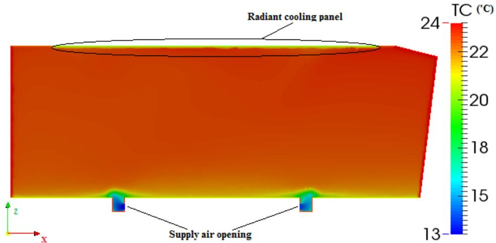
**Figure 69 Predicted temperature distribution near diffusers**
