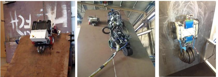
LHS: Advanced wireless wall climbing robot for the inspection of welds on ship hulls. RHS: Magnetic Adhesion Concrete Climber
