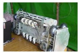
ROBTANK: Mobile in-service robot enters through manholes on the floating or fixed roof of a storage tank to inspect its floor and walls
