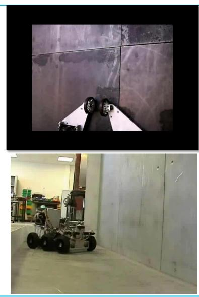
NDT robot adapts to Convex/Concave structures
