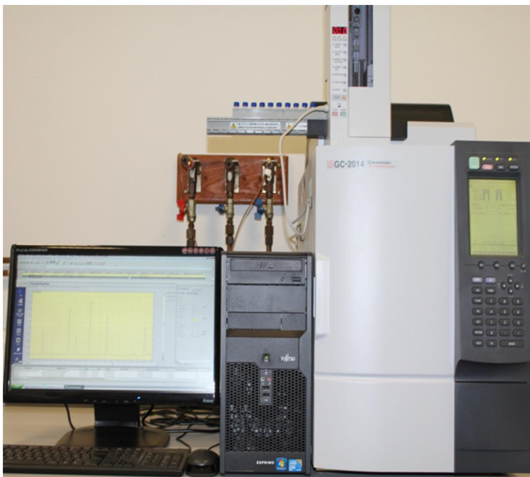
Figure 3.3. A Shimadzu gas chromatography (GC-2014) used for analysis of experimental samples.
