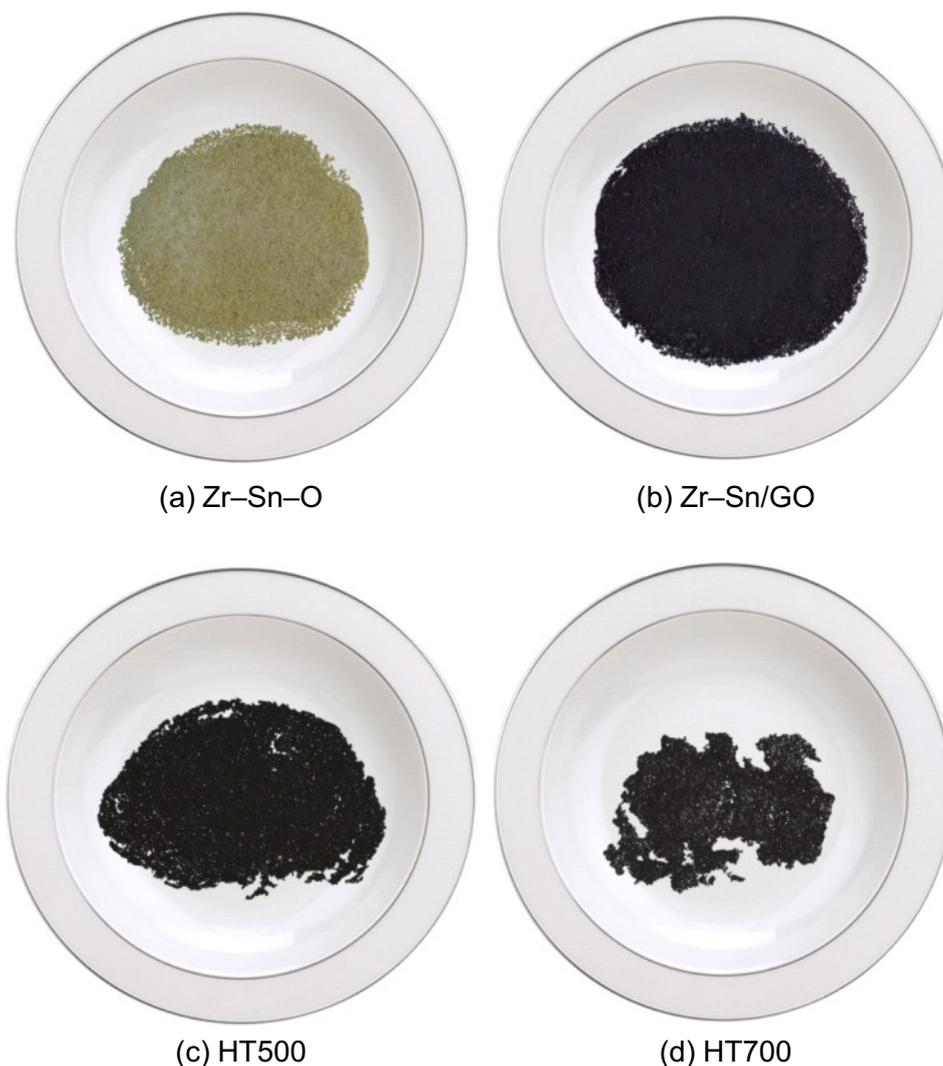
Figure 6.3. Photographic images of tin doped zirconia samples: (a) pure tin doped zirconia as-prepared sample synthesised using CHFS route labelled as Zr-Sn-O; (b) tin doped zirconia graphene nanocomposite as-prepared sample synthesised using CHFS route labelled as Zr-Sn/GO; (c) Zr-Sn/GO heat-treated (773 K) sample labelled as HT500 and (d) Zr-Sn/GO heat-treated (973 K) sample labelled as HT700.
