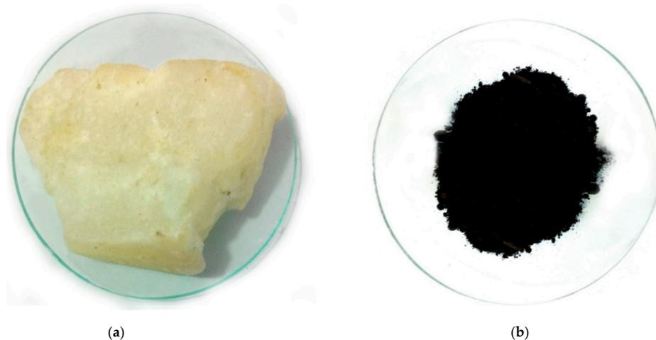
**Figure 2.** Materials used in the present study—(a) paraffin and (b) graphene oxide.
